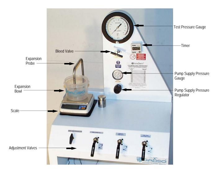
Figure 2- 2 Analog GTC Test Console
