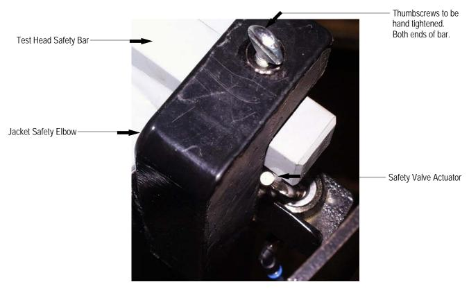
Figure 7-3 Interlock Actuator
