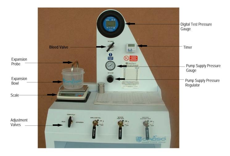
Figure 2- 1 Digital GTC Test Console
