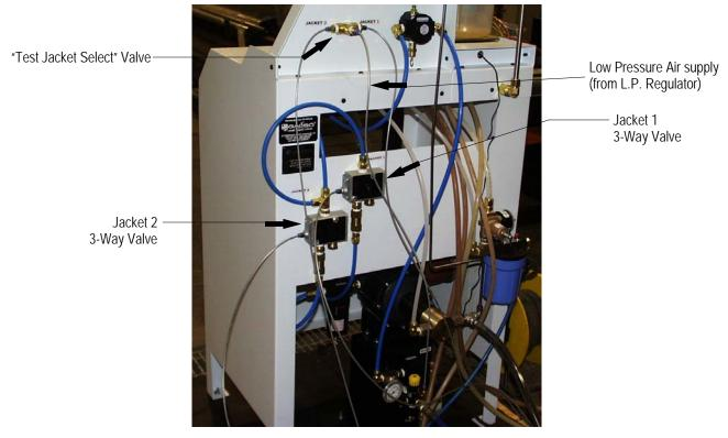
Figure 7-2 Interlock Parts-Rear of Console
