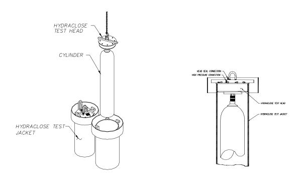
Figure 5 - 1 Cylinder/Test Head Installation
