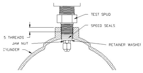
Figure 3 - 1 Hydraclose Seal
