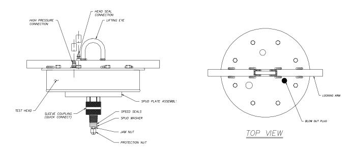
Figure 4 - 5 Hydraclose Test Head
