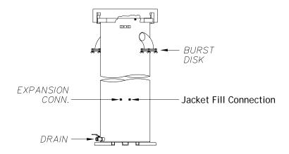
Figure 4 - 4 Hydraclose Test Jacket
