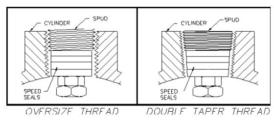
Figure 3 - 2 Cylinder Neck Thread Detail
