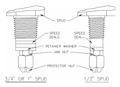
Figure 4 - 6 Speed Seal Details
